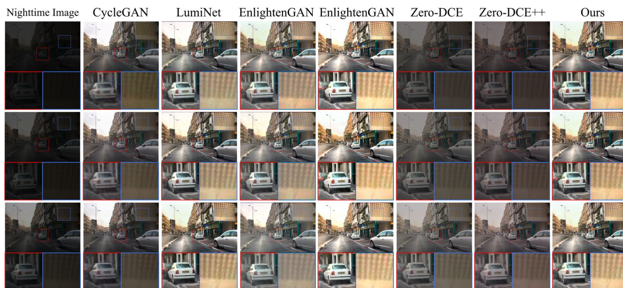
Figure 10. Image enhancement results of each method under different illumination intensities.
