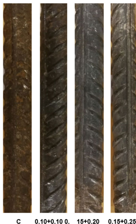
Figure 10. Digital images of mortars embedded rebars retrieved after 43 cycles of wet/dry treatments.
