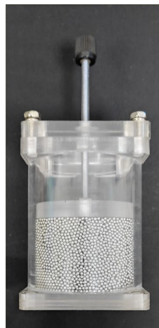
Figure 3. Granular assembly container schematic diagram.
