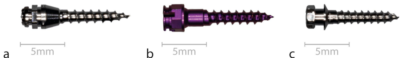
Figure 2. Examined miniscrews. (a) tomas-pin SD N 08 (Dentaurum, Ispringen, Germany). (b) OrthoEasy Pin (Forestadent, Pforzheim, Germany). (c) Dual Top G2 (Promedia, Siegen, Germany/Jeil Medical, Seoul, Republic of Korea).
