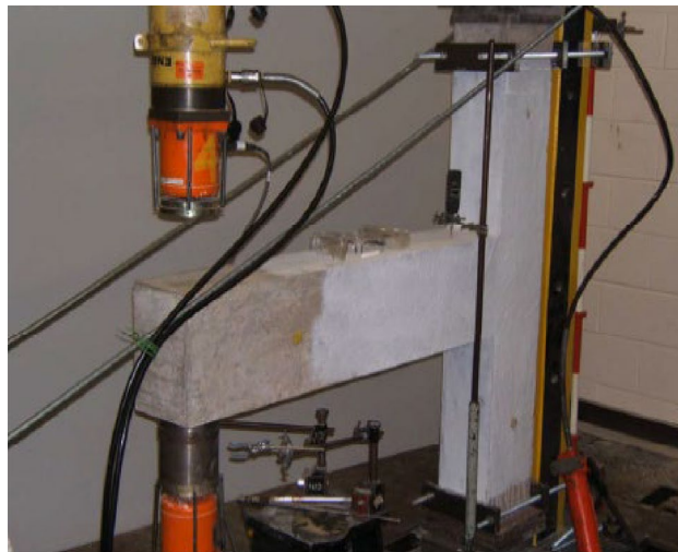
Figure 4. Beam column joint Before loading.
