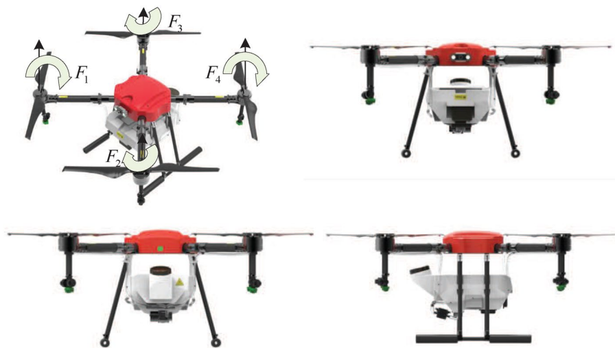
Figure 1. The structure diagram of a QUAUV.
