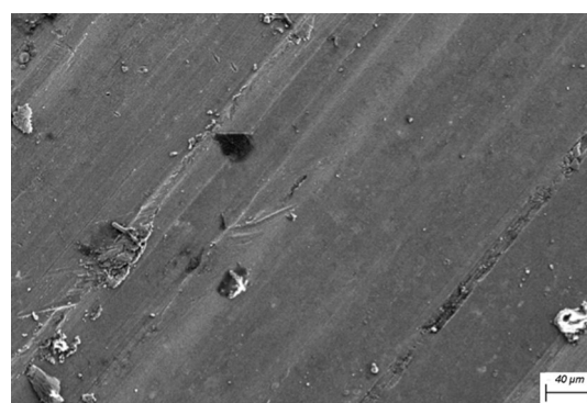
Figure 22. FE-SEM image of the specimen worn surface at the optimum condition of 10 N, 500 m, 1 m/s.
