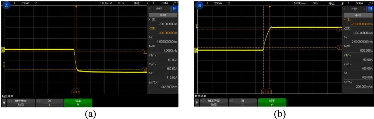
Fig. 10. The dynamic performance of the battery emulator. (a) -50 A — -450 A. (b) 50 A — 450 A.
