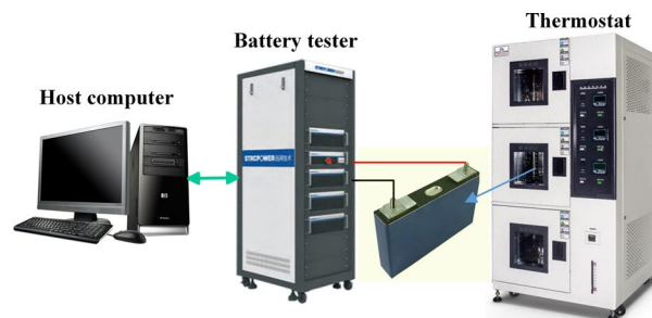
Fig. 5. The battery test bench in this work.
