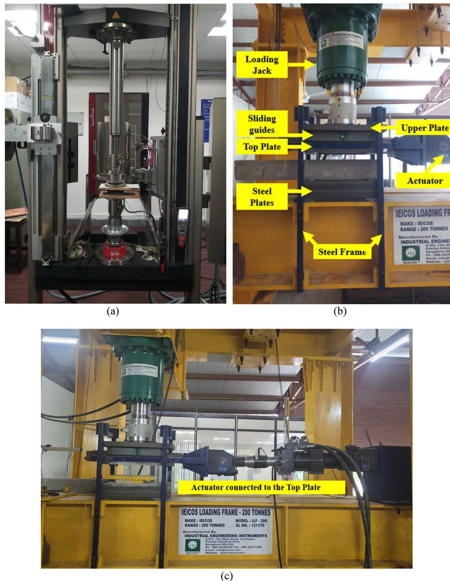
Fig. 2. (a) Zwick Z100 UTM, (b, c) arrangement for Shear cyclic test.
