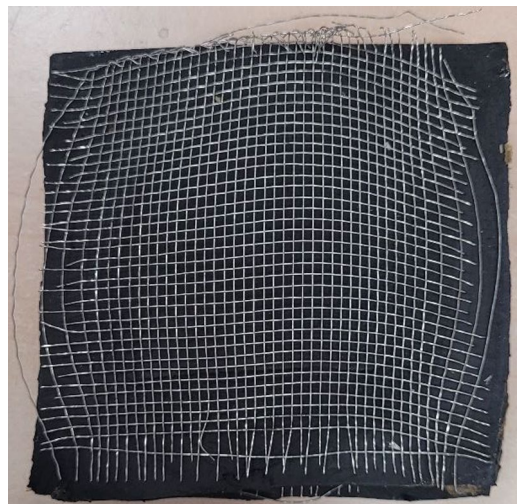
Fig. 9. Debonding of the steel mesh wire.
