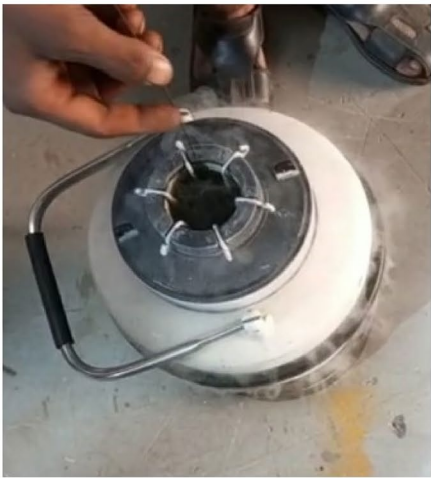
Tool dipped in liquid nitrogen container for 24 hrs.
