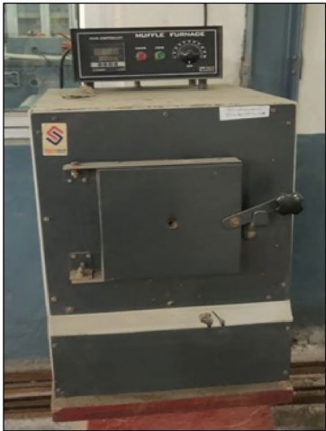
Heating furnace used to heat tool at 600 degree Celsius.
