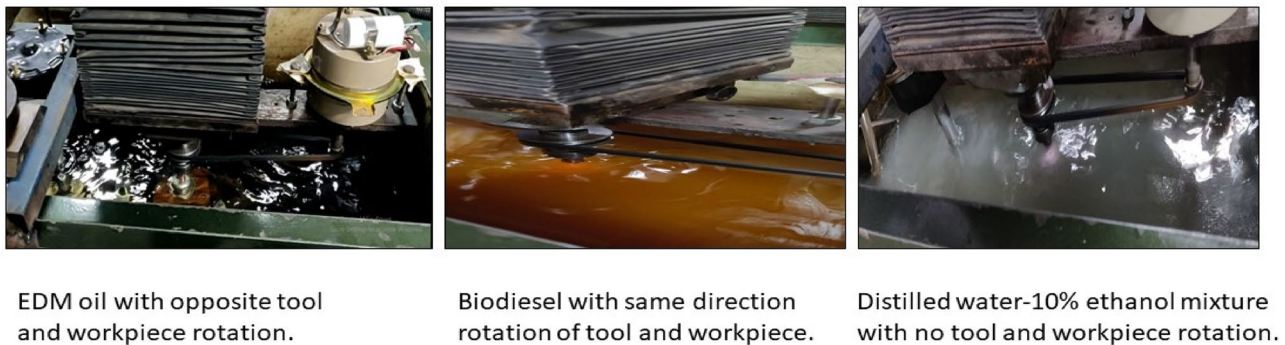
Fig. 12. Shows EDM using different dielectrics as well as different rotation of tool and workpiece.
