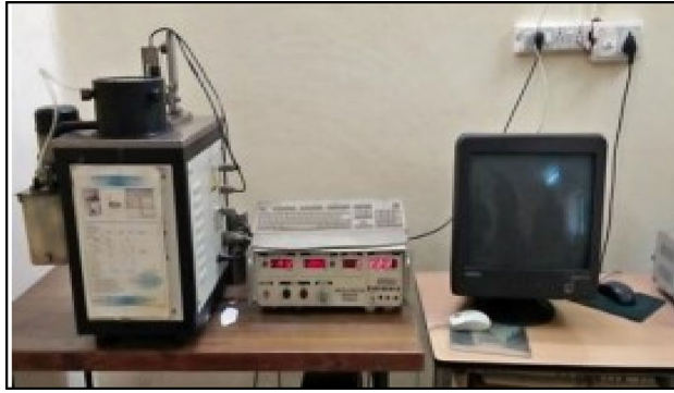
Fig. 10. Shows Pin on disc wear tester.
