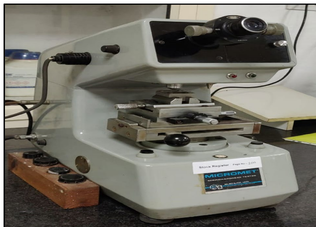
Fig. 9. Shows the microhardness testing machine.
