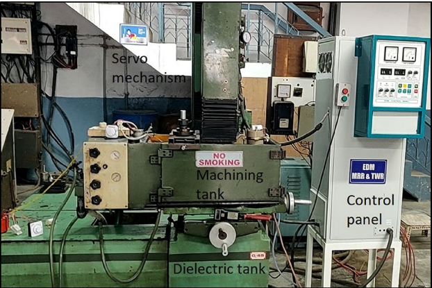
Fig. 3. Depicts the Electric discharge machine used in the experiment.
