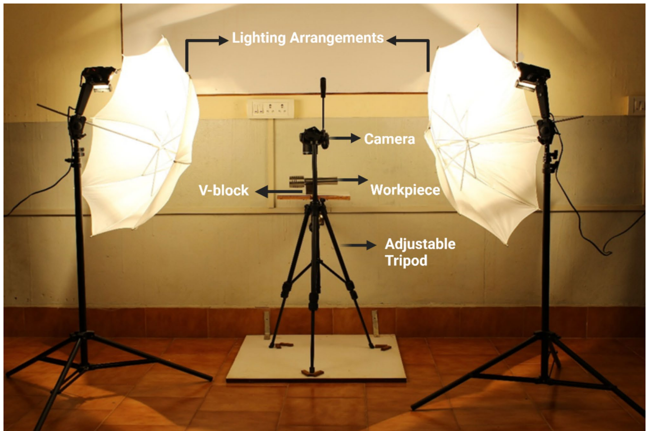
Fig. 3. A simple computer vision setup for capturing turned images.
