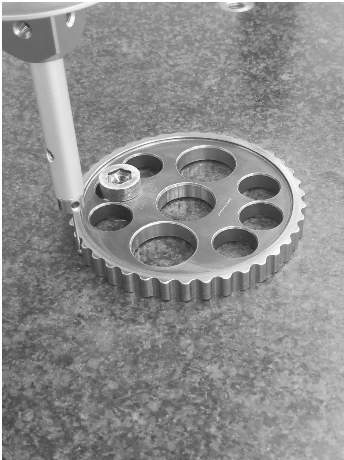
Fig. 8. Physical diagram of cycloidal wheel.
