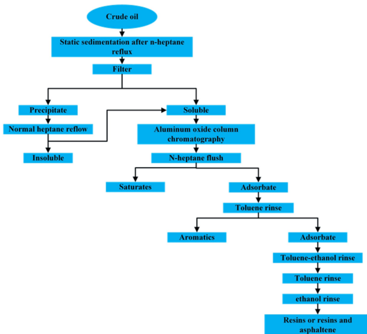
Fig. 2. Detailed separation process of Saturates, aromatics, resins, and asphaltenes.
