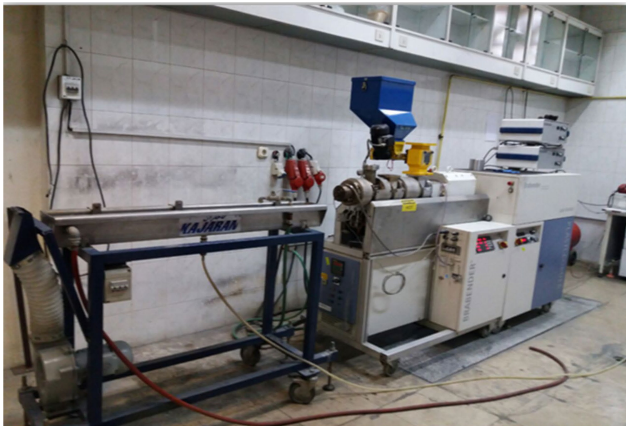
Fig. 2. Twin Screw counter-current extruder to produce CFRP composite.
