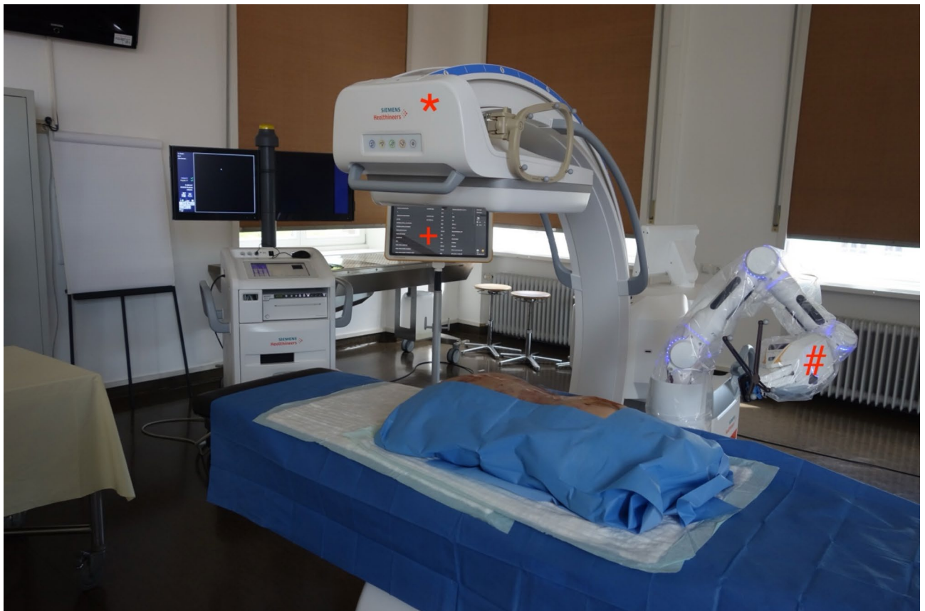
Fig. 1. Experimental set-up: *, 3D-C-arm, #, robotic arm, +, navigation display cart.
