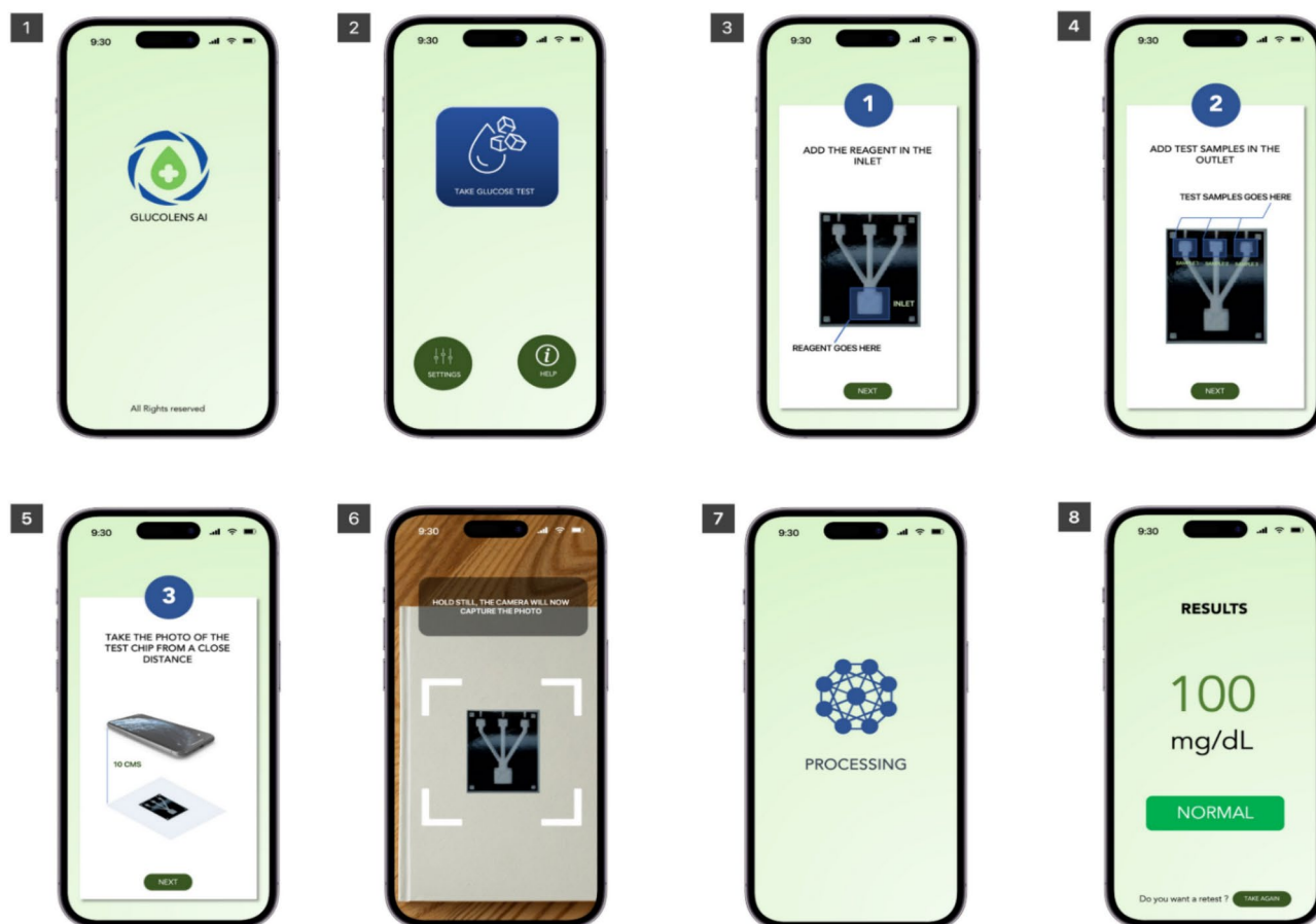
Fig. 8. The various stages of digital glucose colorimetric estimation using the “GLUCOLENS AI” smartphone application. In Fig. 1. The application opening stage, 2. The Home page to initiate the glucose test with settings and information buttons, 3. Placing reagent in inlet well, 4. Adding glucose test samples to outlet wells, 5. The application asks the user to place the smartphone camera on top of the device at well-defined distance, 6. The application captures the image of the test device, 7. Processing page and 8. Result display page.
