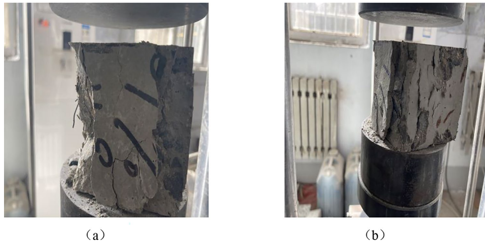
Fig. 5. After 100,000 cycles of load, the compressive strength damage pattern was observed.
