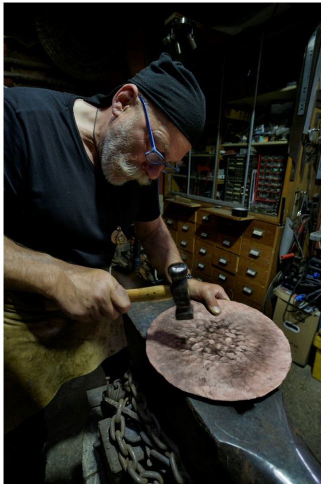
Fig. 4. The copper smith (Herbert R. Bauer) producing a replica of the Nebra Sky Disc by helical hammer forging ((c) State Office for Heritage management and Archaeology, Saxony-Anhalt—State Museum of Prehistory, photo: J. Lipták, Munich).
