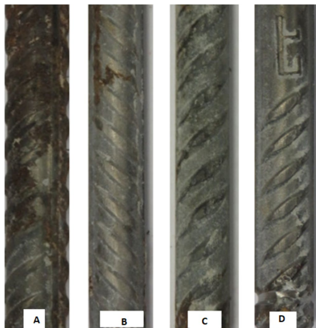
Fig. 8. Images of rebars embedded in the control (A), 0.0625% GA (B), 0.125% GA (C), and 0.25% GA (D) mortars after 37 cycles of wet/dry treatment.
