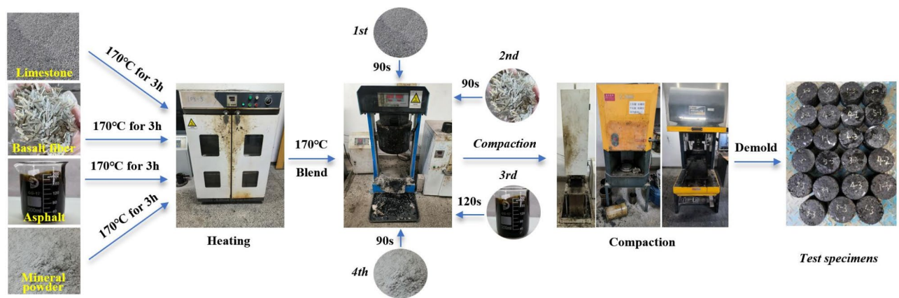
Fig. 4. Production process of mixtures specimens.
