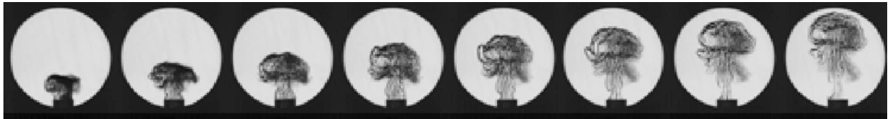
Fig. 5. The schlieren diagram of the flame propagation process of coal dust explosion with a concentration of 350 \text{ g/m}^3 at the tube outlet, particle size less than 53 \mu\text{m} .
