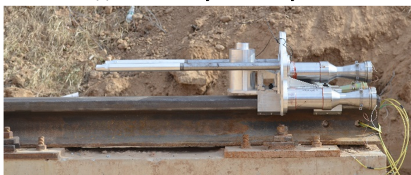
(b) Arrangement of the rocket sled in the experiment
