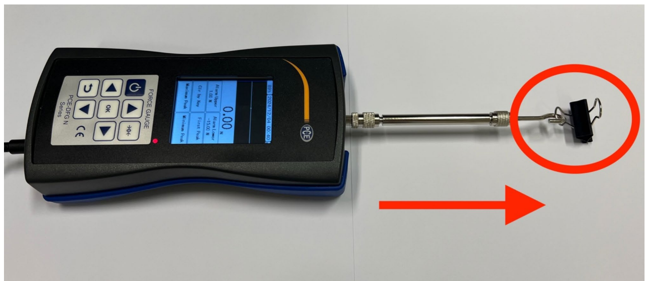
Fig. 6. The tensiometer set up. Direction of applied force is indicated by the red arrow. The clamp which crasped the IOL at the center is marked by the red circle.
