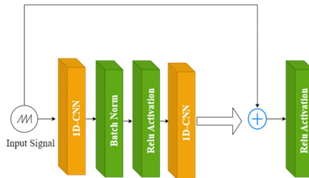
Fig. 4. Architecture of the residual block used in the modified ResNet34 model for PPG signal analysis, showing the flow of data through 1d-CNN layers, batch normalization, and ReLU activation, with a skip connection to combat the vanishing gradient problem.
