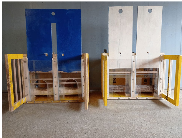
Fig. 1. Left, joint log-lift (JLL) box with front panel open and log fully down. Right, individual log-lift (ILL) box with both front panels open and both logs fully down.
