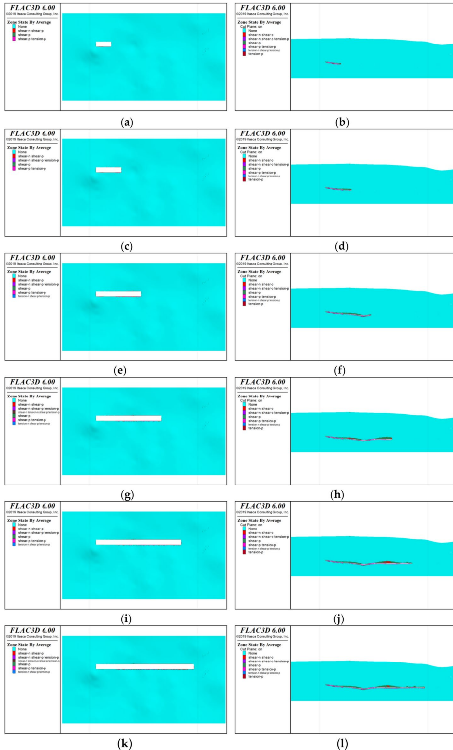
Fig. 20. The distribution of the plastic zone of the surrounding rock during the mining process of the 1802 working face: (a) Plane plastic zone distribution after 600 m excavation; (b) Profile plastic zone distribution after 600 m excavation; (c) Plane plastic zone distribution after 1000 m excavation; (d) Profile plastic zone distribution after 1000 m excavation; (e) Plane plastic zone distribution after 1800 m excavation; (f) Profile plastic zone distribution after 1800 m excavation; (g) Plane plastic zone distribution after 2600 m excavation; (h) Profile plastic zone distribution after 2600 m excavation; (i) Plane plastic zone distribution after 3400 m excavation; (j) Profile plastic zone distribution after 3400 m excavation; (k) Plane plastic zone distribution after 3900 m excavation; (l) Profile plastic zone distribution after 3900 m excavation.
