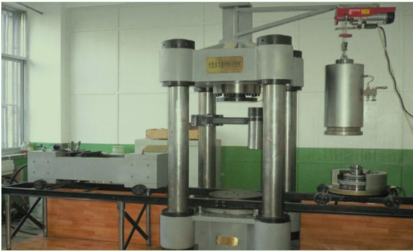
Fig. 3. WDT multifunctional material testing machine.
