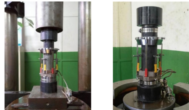
(a) Uniaxial compression test (b) Triaxial compression test
