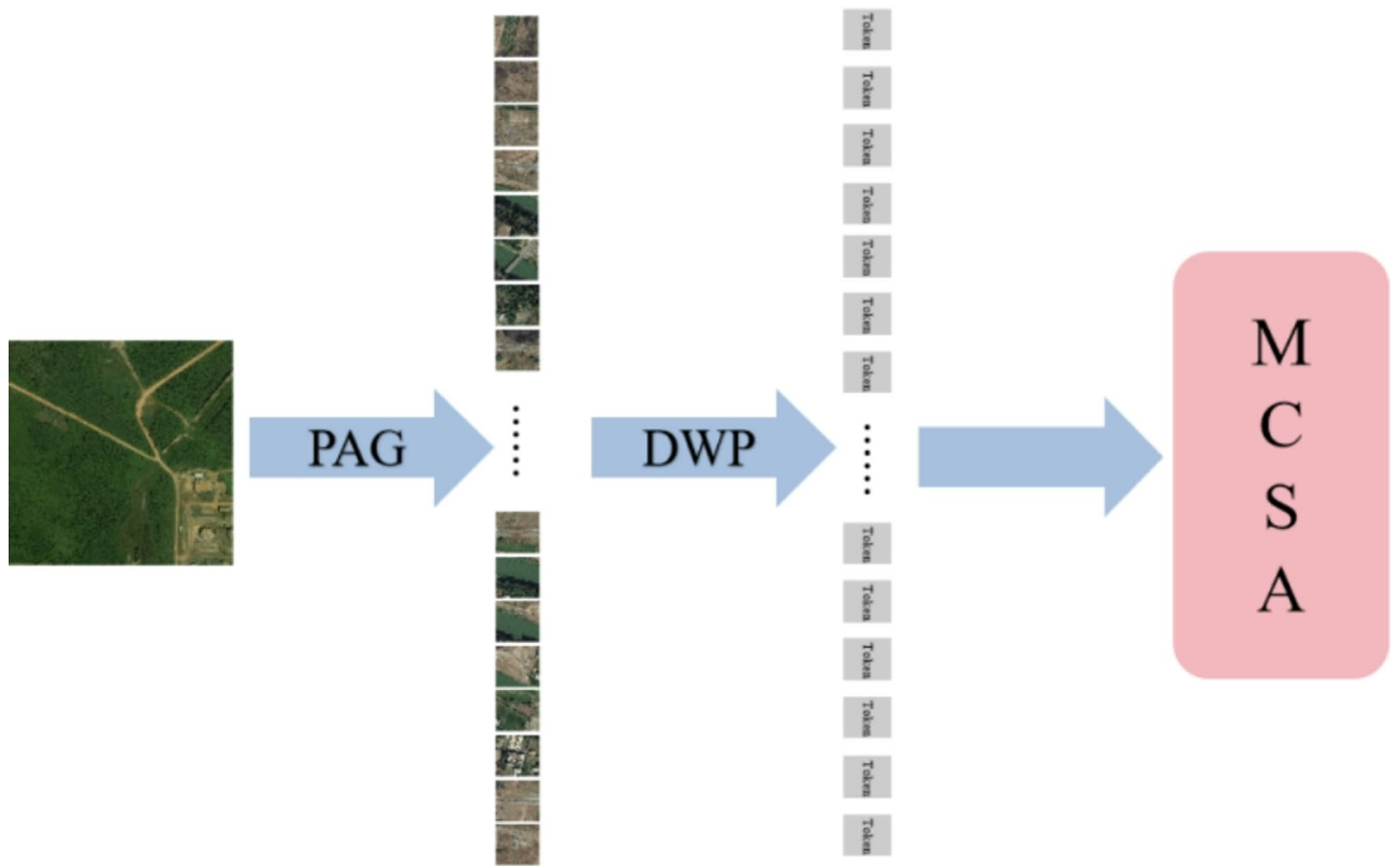
Fig. 5. Input a 512*512 remote sensing road image, after PAG module, the image is averagely cut into N small images, and then these images are transformed into T embedded vectors through DWP module, and finally these embedded vectors are passed into MCSA. Satellite images were generated using the DeepGlobe Road Dataset under CC BY 4.0.
