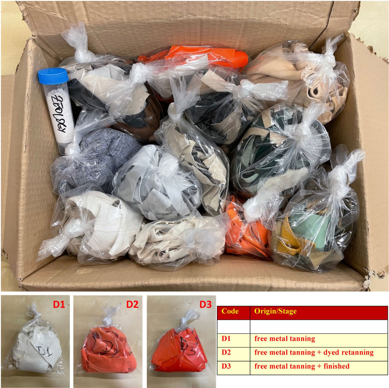
Fig. 1. Photograph of processing wastes as received from the tannery, at the top. Photos of the distinct classified materials, at the bottom.
