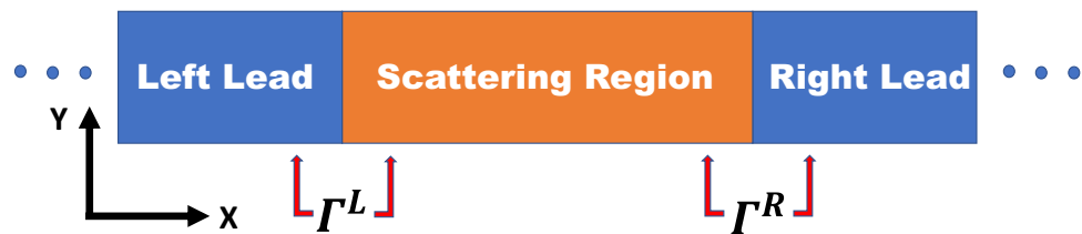
Fig. 9. A schematic diagram for two terminal device (scattering region connected with two infinite leads).
