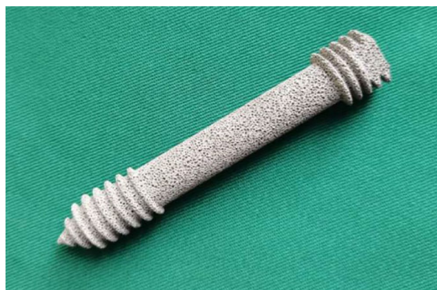
Fig. 1. The external morphology of porous tantalum metal screws.
