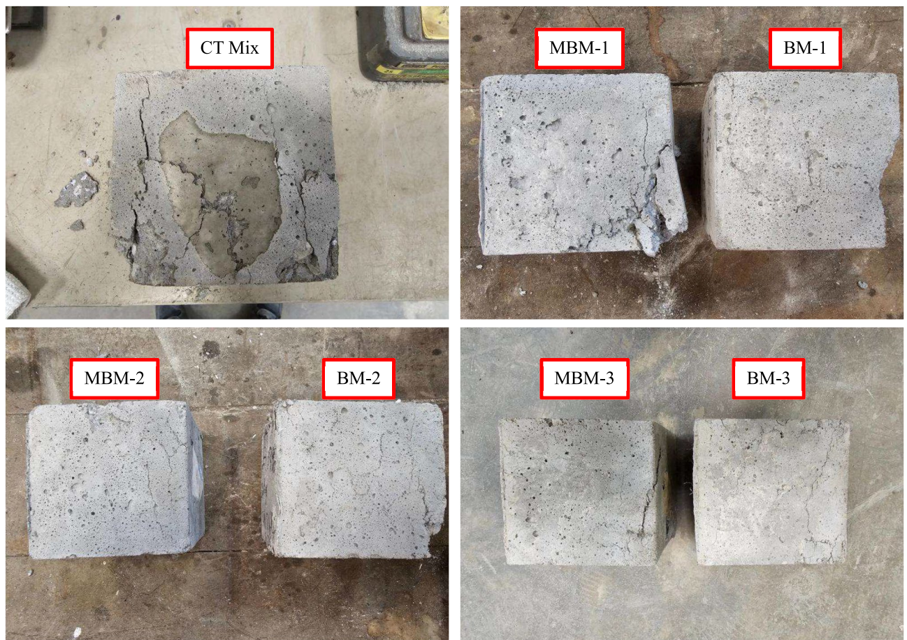
Fig. 10. Failure mode of the concrete cube after loading.
