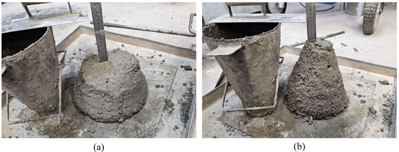
Fig. 7. Effect of fibre addition on concrete workability: (a) without fibre, (b) with 0.3% fibre.
