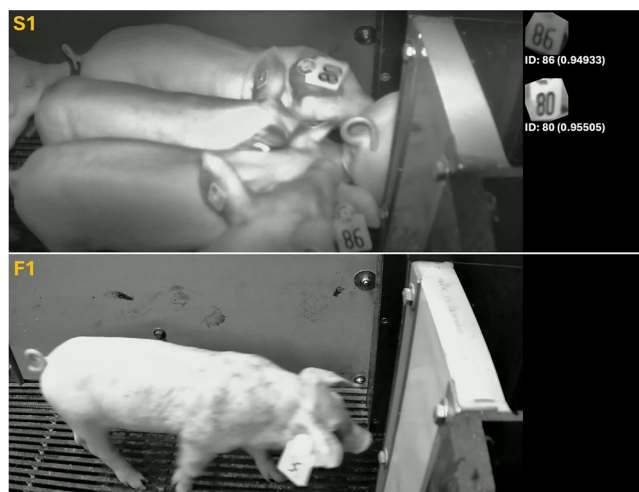
Fig. 8. Example frames of a successful (S1) and a failed ID identification (F1) taken from Use Case 2. (S1) On the right side, two ear tag crops with ID proposals and confidence values in parentheses below the crop are shown. (F1) The ear tag with ID 96 was not detected due to a combination of overexposure of the image and motion blur of the animal.
