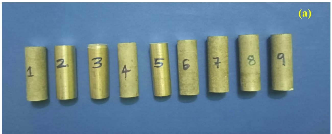
Fig. 1. (a) Tribological testing Al7075-WC composite samples. (b) Qualitative result and EDS of Al7075-WC composite samples at different positions from the parent composite. (c) SEM and EDS of tungsten carbide reinforcement in the composite samples. (d) Particle size of Tungsten Carbide.
