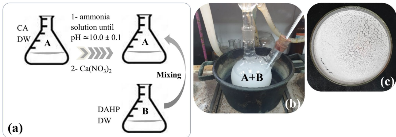
Fig. 3. Schematic diagram illustrates the preparation of synthetic hydroxyapatite (SHA). (a) Mixing of the chemical components; (b) The resulting solution was placed in a water bath at 70 °C and stirred for 24 h; (c) The resulting powder obtained after drying the suspension in a thermostatic drying oven at 60 °C for 4 h.
