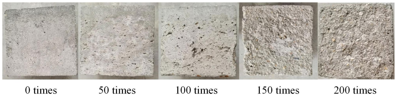
Fig. 4. Surface topography of SCC under different F-T cycles.
