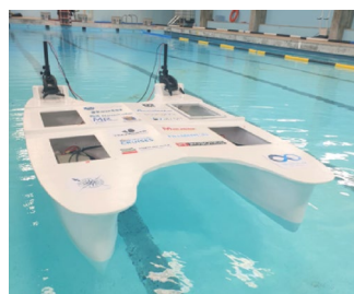
Fig. 1. Unmanned surface vehicle initial prototype.
