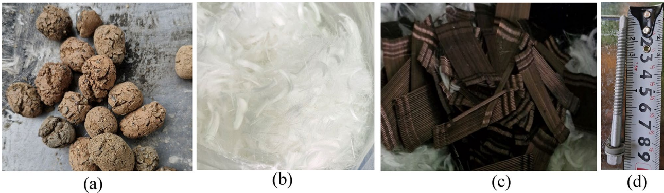
Fig. 2. Lightweight concrete with the proportion of mixed fiber materials: a shape of karemzit lightweight aggregate; b polypropylene fiber; c steel fiber; d screw with a diameter of 5.5 mm.
