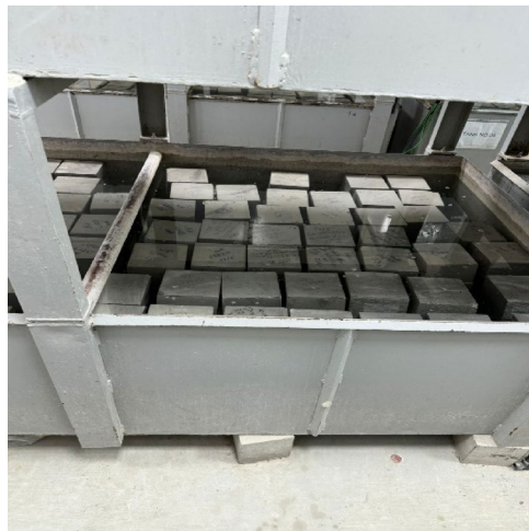
Fig. 4. Temperature-controlled curing tanks.
