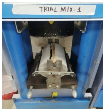
Fig. 8. Sample set in machine to determine splitting tensile strength.
