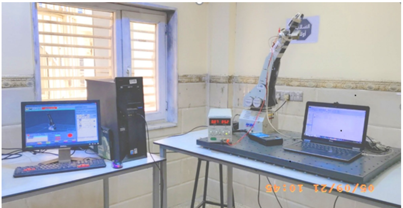
Fig. 2. Work environment for LabVolt 5150 robot arm.
