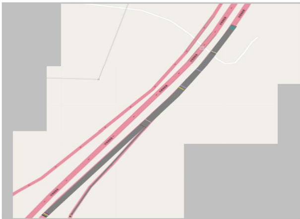
Fig. 3. Detector setup and traffic data capture zones for the interchange entrance of G4 Beijing-Hong Kong-Macao expressway and G45 Daqing-Guangzhou expressway.
