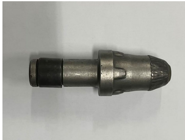
Fig. 3. The physical image of pick used in tests.
