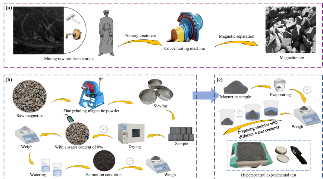
Fig. 1. Experimental flow chart: (a) magnetite collection, (b) magnetite sample treatment and saturation measurement, (c) magnetite spectrum experimental test.
