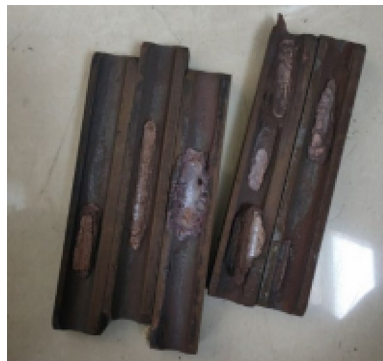
Fig. 1. Carbon brush with heavy carbon accumulation.
