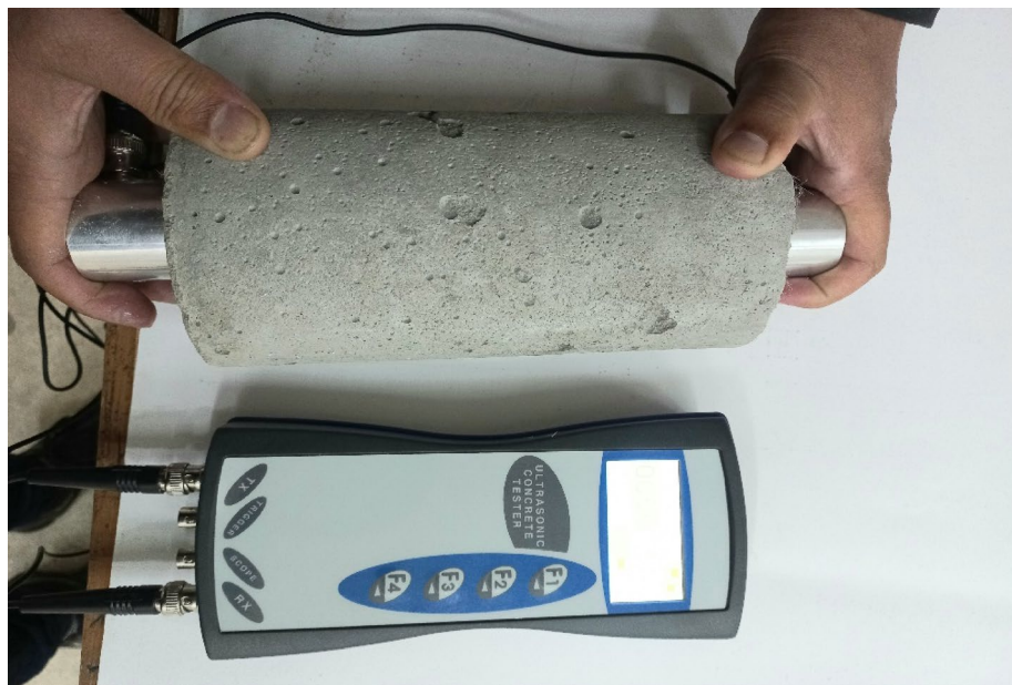
Fig. 19. UPV test of specimen.
