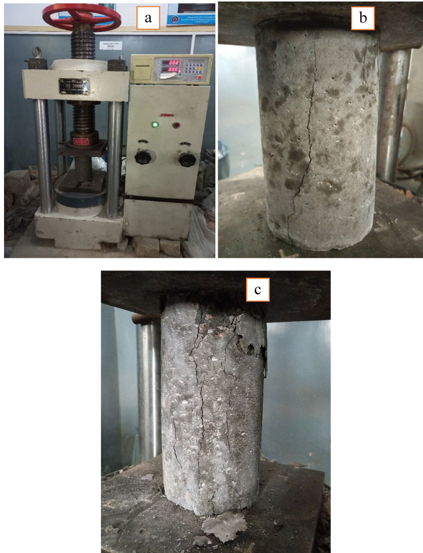
Fig. 7. (a) Specimen under testing machine; (b) Crack in Natural Aggregate Concrete; (c) Crack in Recycled Aggregate Concrete.
