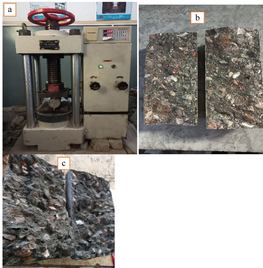
Fig. 10. (a) Specimen under testing machine; (b) Crack in Natural Aggregates Concrete; (c) Crack in Recycled Aggregates Concrete.
