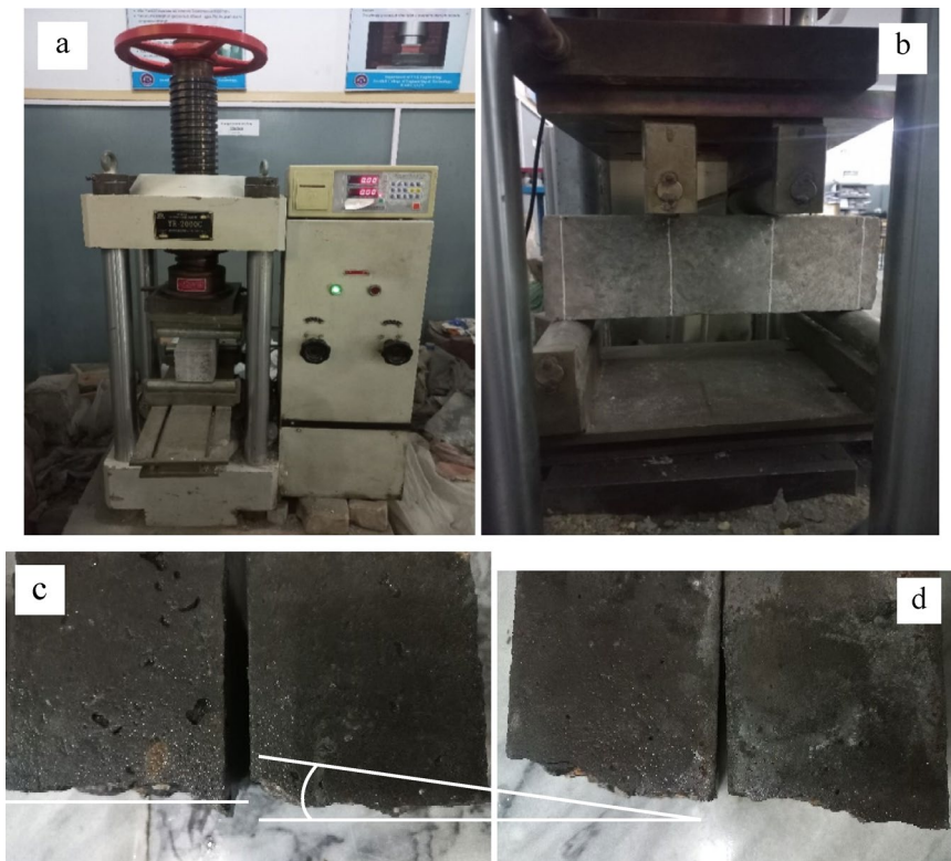
Fig. 12. (a) Sample in Testing Machine; (b) Markings; (c) Linear Cracks in Natural Aggregates Concrete; (d) Diagonal Cracks in Recycled Aggregates Concrete.
