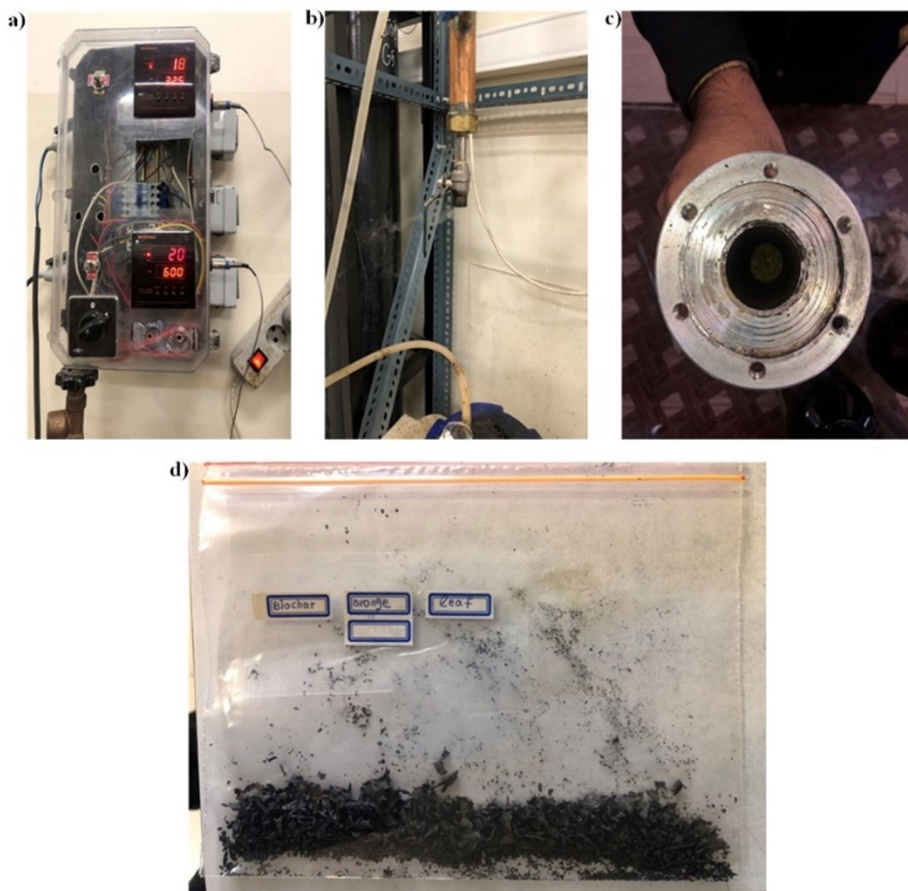
Fig. 3. (a) Pyrolysis of biomass conducted in a nitrogen atmosphere furnace; (b) Release of biogas during the synthesis of MBC-OL; (c) Completion of the MBC-OL synthesis process; (d) Washing and drying of MBC-OL at 85 °C to remove impurities and enhance stability.
