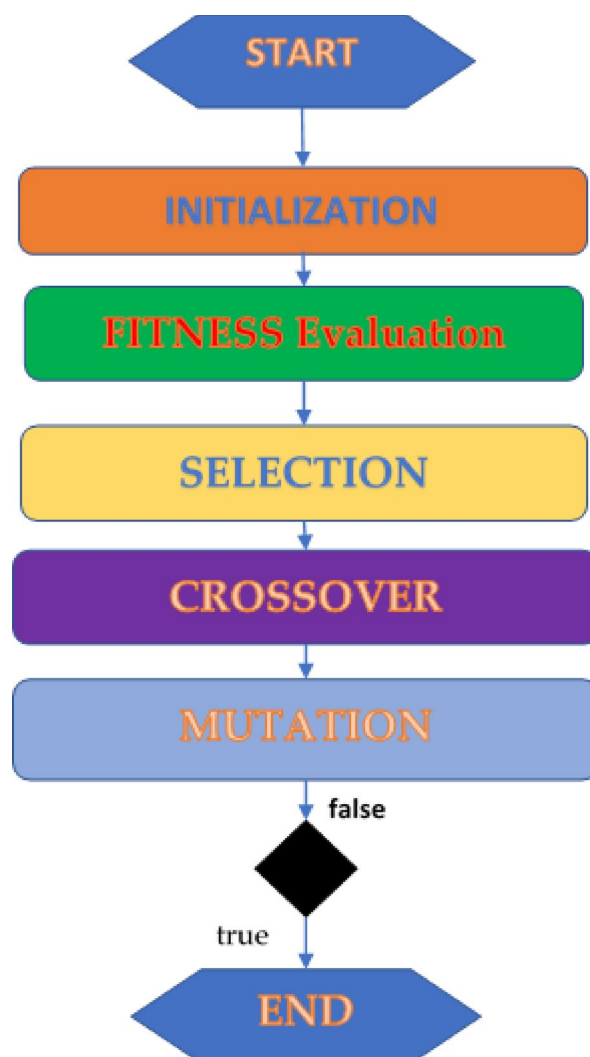
Fig. 2. Flowchart for a genetic algorithm 37 .
