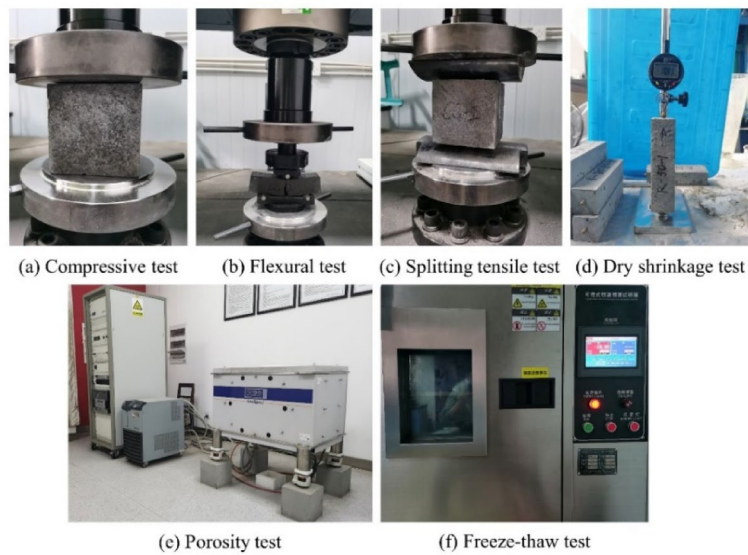
Fig. 4. (a) Compressive test, (b) Flexural test, (c) Splitting tensile test, (d) Drying shrinkage test, (e) Porosity test, and (f) Freeze-thaw test.
