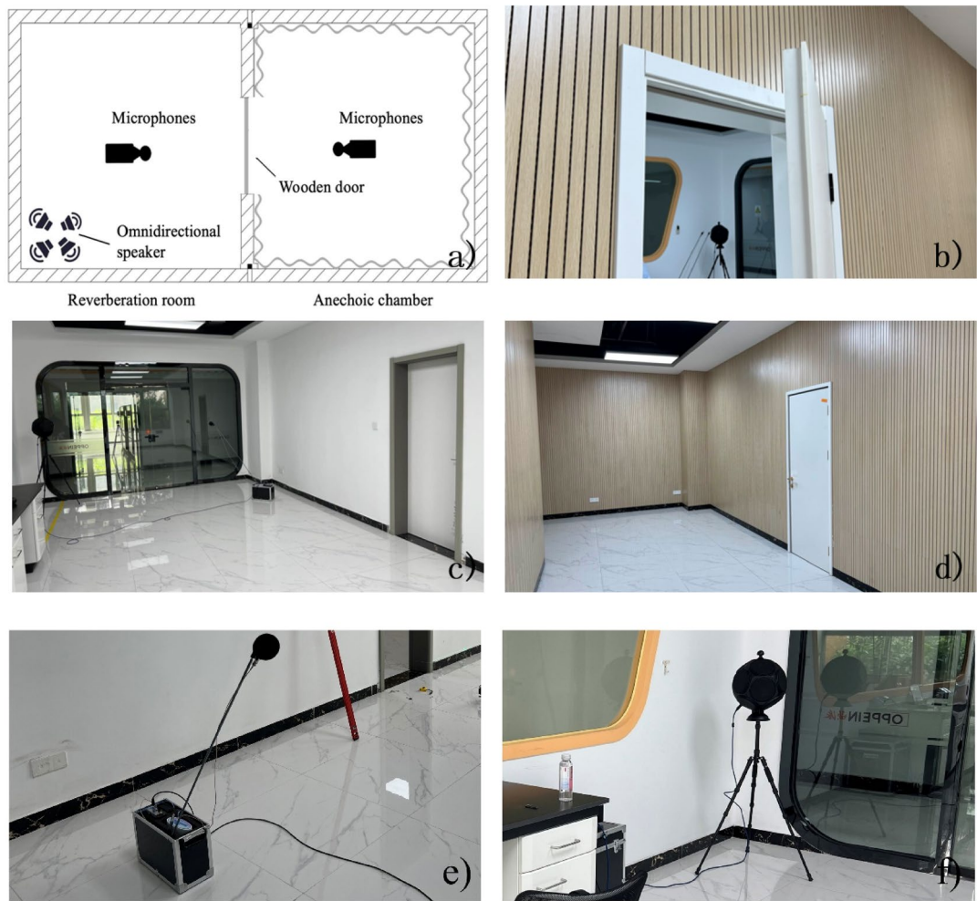
Fig. 3. Reverberation chamber - anechoic chamber dual-chamber method: (a) Schematic diagram of the two-chamber method; (b) Wooden door; (c) Reverberation room; (d) Anechoic chamber; (e) Test AWA 14,423 type condenser microphone; (f) AWA 6021a sound level calibrator.
