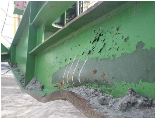
Fig. 9. Exemplary damage after a failure of the carrying structure of the discharge boom—plastic deformation.
